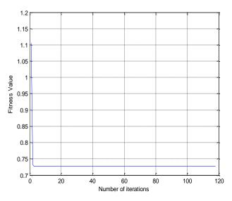
Fig.4Fitness curve for relay coordination of system-2 obtained by PSO technique
